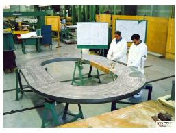
Starting of ground insulation process
