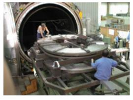
DP4 ready for heat treatment. Superconducting samples of ENEA and FZK in front of top pancake. Incoloy mould frame under the top pancake
